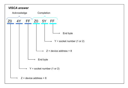
The time between the acknowledgement and the completion packet depends on the command. The answer for an inquiry is Z0 5Y followed by the information requested with FF as end byte.
